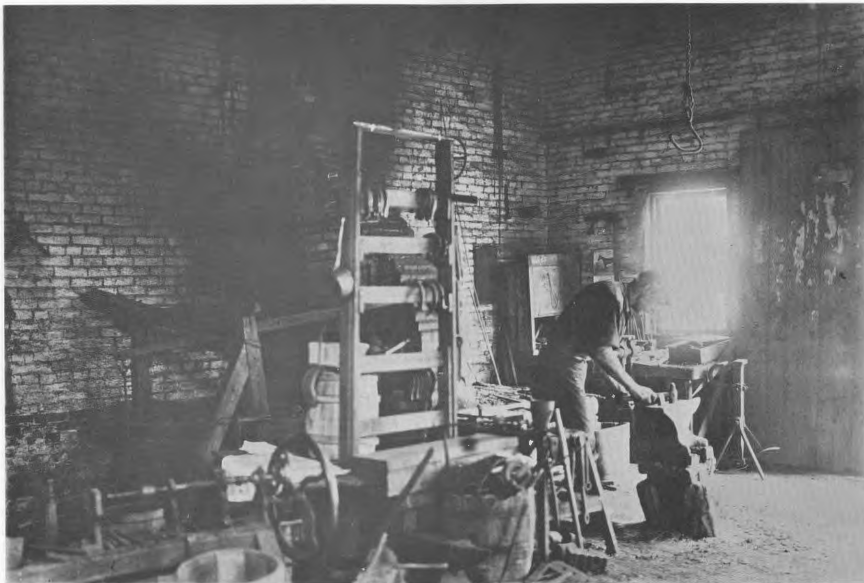
The inside of the blacksmith shop showing the anvil and tools. At the left is the handle for pumping the bellows and the wheel and rod below that is the apparatus for putting the metal rims on wheels for wagons and carriages.
